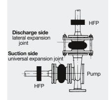
Recommendation for arranging expansion joints at pumps (normal case)
