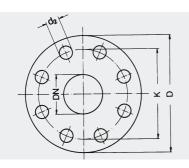
For pipes and fittings the screw holes must be placed in such a way as to be clear of the horizontal and vertical axes.
