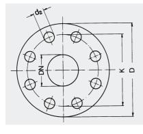
The number of screw holes for every flange is divisible by 4. For pipes and fittings, the screw holes must be placed in such a way as to be clear of the horizontal and vertical axes.
