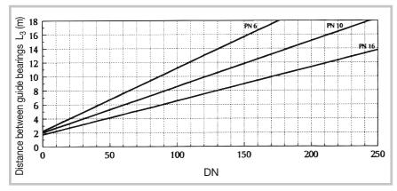
$\begin{array}{lll} L_1 &=& distance \ between \ expansion \\ & joint/pipe \ connector \ and \ fixed \\ & point \ or \ distance \ between \ expansion \\ & joint/pipe \ connector \\ & and \ 1^{\rm st} \ guide \ bearing \\ & (L_1 \leq 3 \ x \ DN) \end{array}$
