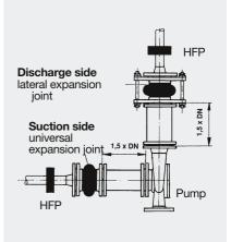
Pumping media with abrasive solid particles (special case)
