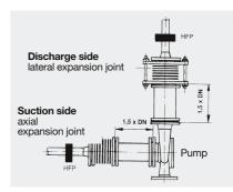
Pumping media with abrasive solid particles (special case)
