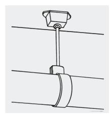
Pendulum-type pipe suspensions are not fixed points
