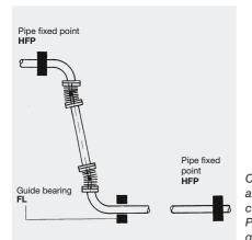
As a rule only one compensation system may be placed between two fixed points. When several compensation systems are fitted into the pipe system, fixed points must be provided between them.
