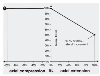
Restriction of the lateral movement with simultaneous axial movement (universal expansion joints)
