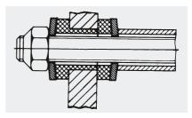
Tie rod restraints are carried in rubber sockets for sound absorption up to DN 150 as a standard feature
