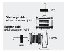
Recommendation for arranging expansion joints at pumps (normal case)
